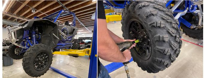
3. Remove the top radius rods first by removing the top nuts and bolt on both ends of the radius rods. To do this, remove the chassis side radius rod bolt with nut and the radius rod hub side nut. Please see the attached image showing location of the bolt.
