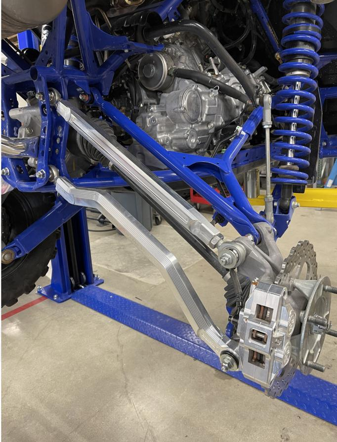
**NOTE:** Ensure that side of the radius rod with the part number engraving is toward the trailing arm side.
