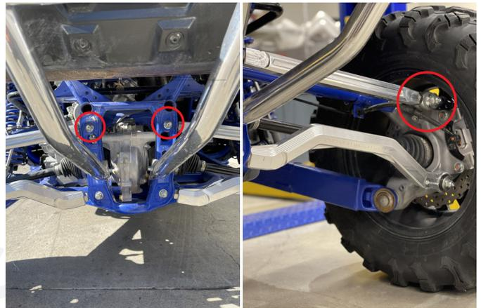
4. Once the radius rod is removed, adjust the length of the PM Off-Road radius rods heim joints. To do this, place two bolts through the OEM radius rods and loosen or tighten the heim joints on the PM radius rods. Adjust the heim joints so that there is an **equal number of threads exposed** on each side of the radius rods. Depending on your UTV model, tightening the jam nut may be easier before installing on your vehicle.
