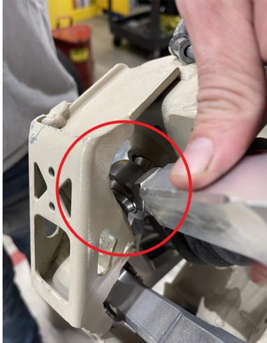
**Note:** Ensure that the P/N engraving is on the same side as the trailing arm side. The top radius rod is the shortest length.
