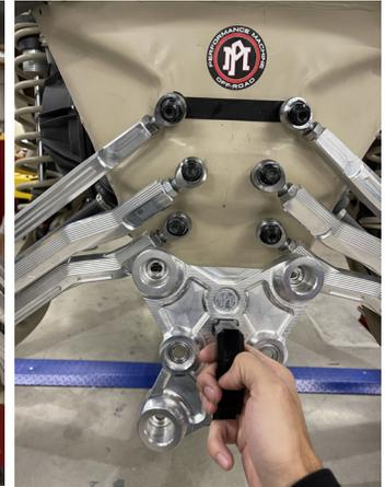
4. Remove the OEM upper radius rods first by unbolting the hub-side bolt.
