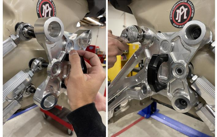
7. Repeat Step 4 and 5 for the remaining PM Off-Road Radius Rods and install the radius rods one at a time.
