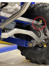
4. Once the radius rod is removed, adjust the length of the PM Off-Road radius rods heim joints. To do this, place two bolts through the OEM radius rods and loosen or tighten the heim joints on the PM radius rods. Adjust the heim joints so that there is an **equal number of threads exposed** on each side of the radius rods. Depending on your UTV model, tightening the jam nut may be easier before installing on your vehicle.
