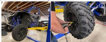
3. Remove the top radius rods first by removing the top nuts and bolt on both ends of the radius rods. To do this, remove the chassis side radius rod bolt with nut and the radius rod hub side nut. Please see the attached image showing location of the bolt.
