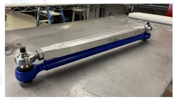
Note: Ensure to use the correct PM Off-Road radius rods when replacing the OEM rods. Please refer to the part number and description engraved on the radius rods and refer to this installation sheet. Use thread locker on all non-nylon hardware and torque to OEM specification. Please refer to your vehicle's owner's manual for exact torque specification.
