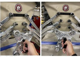
4. Remove the OEM upper radius rods first by unbolting the hub-side bolt.
