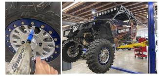
3. Remove the 6 nuts on the chassis brace and remove the OEM radius rod plate. To prevent the radius rods from coming off the studs, temporarily hand screw the nuts to keep them in place.
