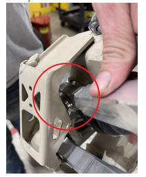
Note: Ensure that the P/N engraving is on the same side as the trailing arm side. The top radius rod is the shortest length.
