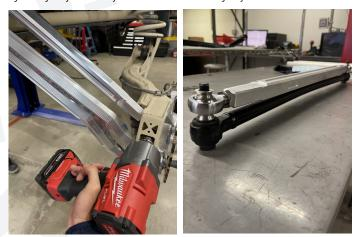
Note: Ensure to use the correct PM Off-Road radius rods when replacing the DEM rods. Please refer to the part number and description engraved on the radius rods and refer to this installation sheet. Use thread locker on all non-nylon hardware and torque to OEM specification. Please refer to your vehicle's owner's manual for exact torque specification.
